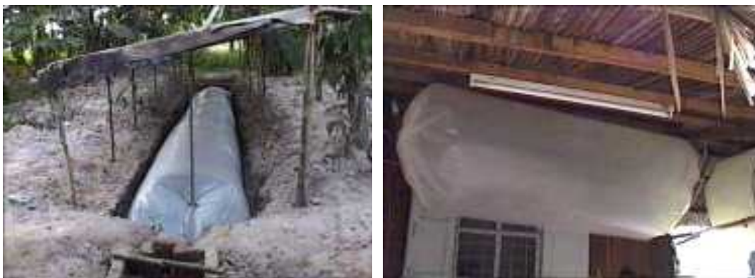
Figure 6. Layer bags (left) and gasholder bag (right) of tube polyethylene biogas digester. Photos by L. Rodriguez.
